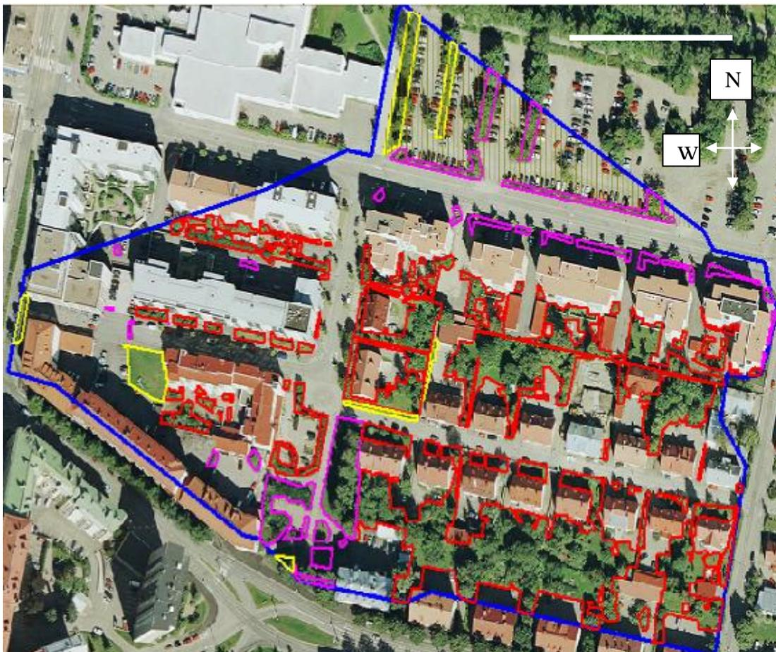
Figure 4. Medium-density catchment area (Paavola) in an urban/suburban area in the City of Lahti. In this figure blue line indicates the border of the catchment. Areas inside red (urban park), magenta (bushes) and yellow (lawn) lines are pervious soils. The white bar at the upper right corner = 100 m.
