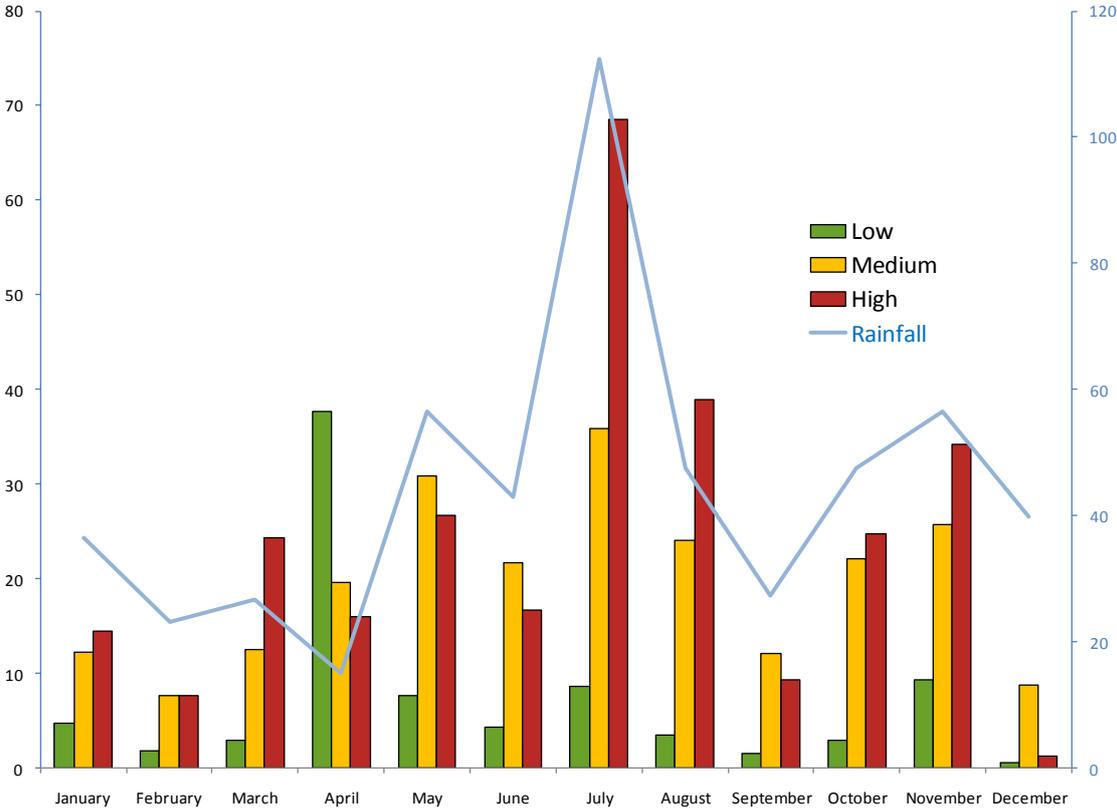
Figure 12. Monthly precipitation (rainfall) (mm; illustrated by the line; right-hand vertical axis) and urban runoff (mm; illustrated by the left-hand vertical axis) at the three catchments with different land-use intensities (low-, medium-, and high-intensity areas) in 2009.
