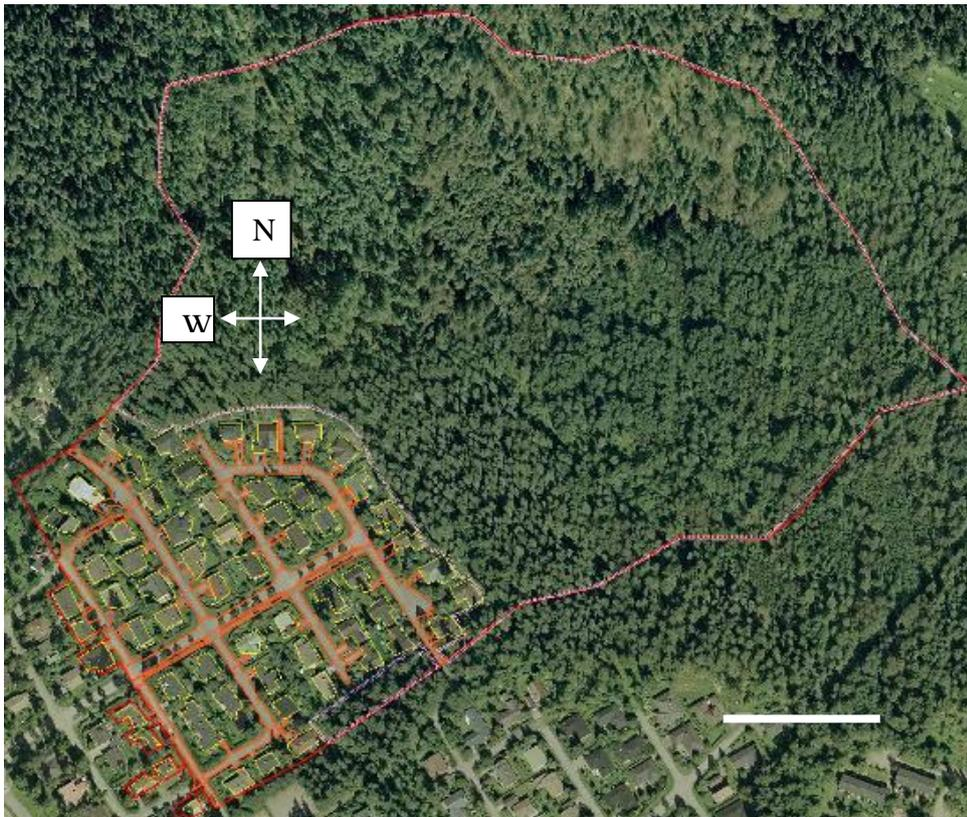
Figure 3. Low-density catchment area (Kilpiäinen) in a rural/residential area in the City of Lahti. The catchment border is illustrated by a magenta/red line. Areas within yellow lines are roofs. Streets and other impervious surfaces on the ground are marked with an orange line. The white bar = 100 m.
