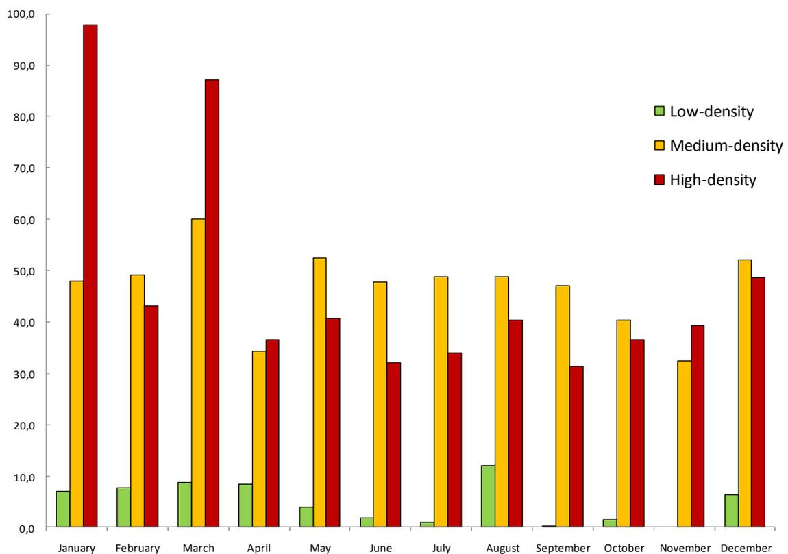
Figure 13. Monthly means (2009) of stormwater conductivity (mS/s) at the three catchments of differing (low-, medium-, and high-density) land-use intensity.
