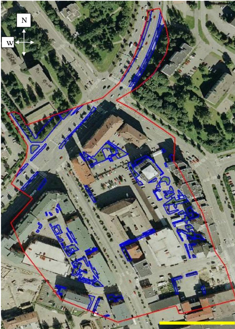
Figure 5. High-density catchment area (Taapelipolku) in the city core of Lahti. Red line indicates the border of the catchment and areas inside blue lines are pervious surfaces. The yellow bar at the low right corner = 100 m.
